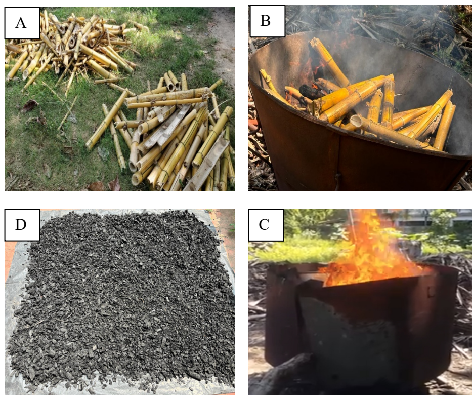
Figure 1. Pyrolysis process using Kon Tiki Biochar Kiln: collection of bamboo culms (A), pyrolysis process at 600°C using Kon Tiki Biochar Kiln (B), clean flames with minimal smoke emission (C) and bamboo biochar (D).
