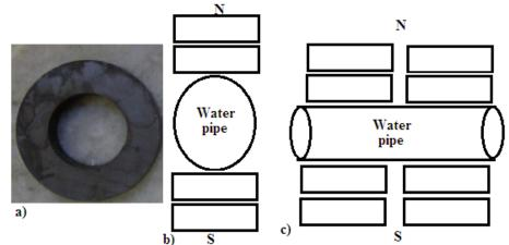
Figure 1 - a) Magnet; b) front view of pipeline containing water; and c) lateral view of vessel containing water.
