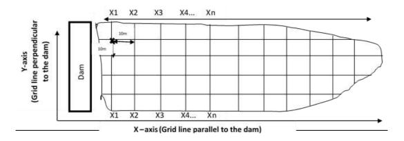
Figure 3 - A plan view of the gridded reservoir for canoe navigation and data acquisition
