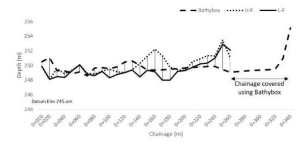
Figure 10 - Reservoir depth profile from Bathybox, Echo Sounder High and Low Frequencies
