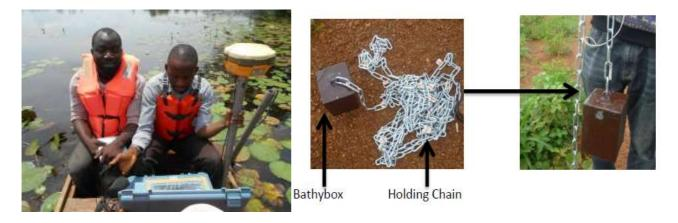
Plate 1- Field set up with Echo Sounder and BATHYBOX
