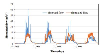
Figure 4 - Daily simulated flow and observed during (a) calibration (1995 – 2002) and (b) validation (2003 - 2006) periods
