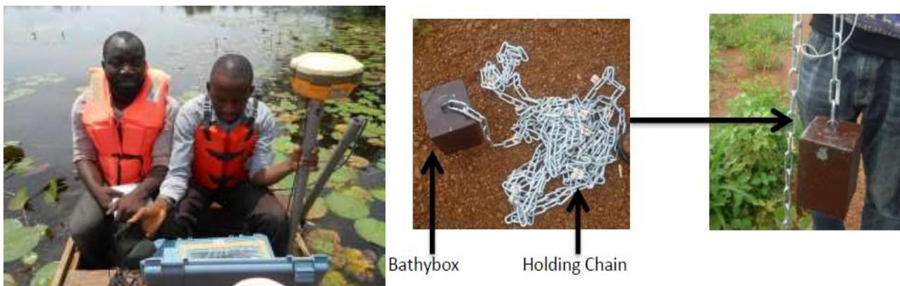
*Plate 1- Field set up with Echo Sounder and BATHYBOX*
