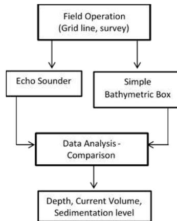
Figure 2 - Protocol for the survey operations
