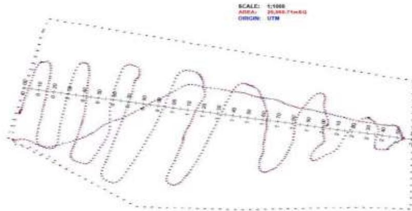
Figure 5 - Survey navigation path for Echo Sounder
