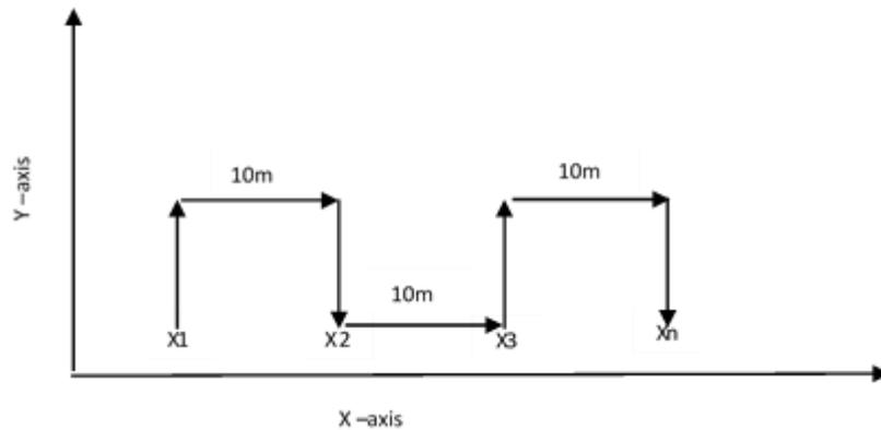
Figure 4 - Movement of the canoe along and across the reservoir
