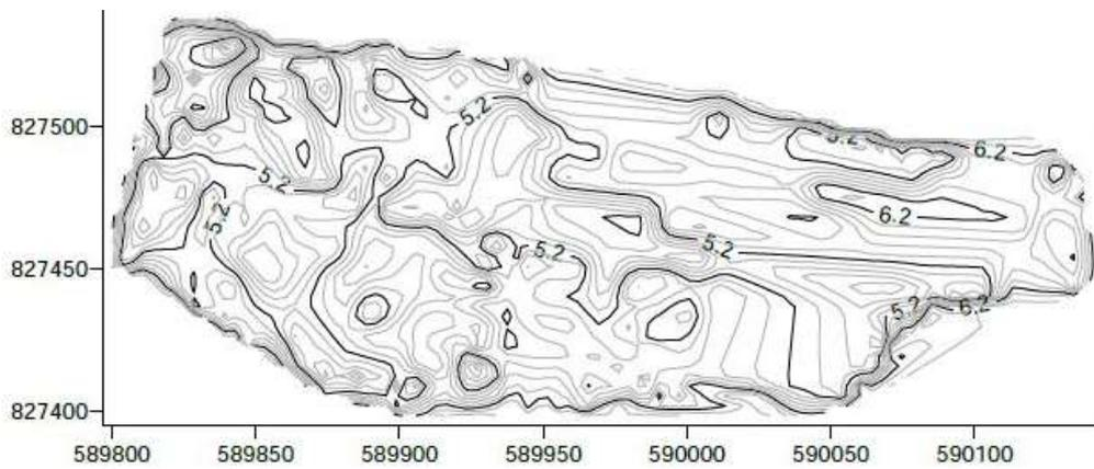
Figure 9 - Contour map generated from the processed bathymetric data
