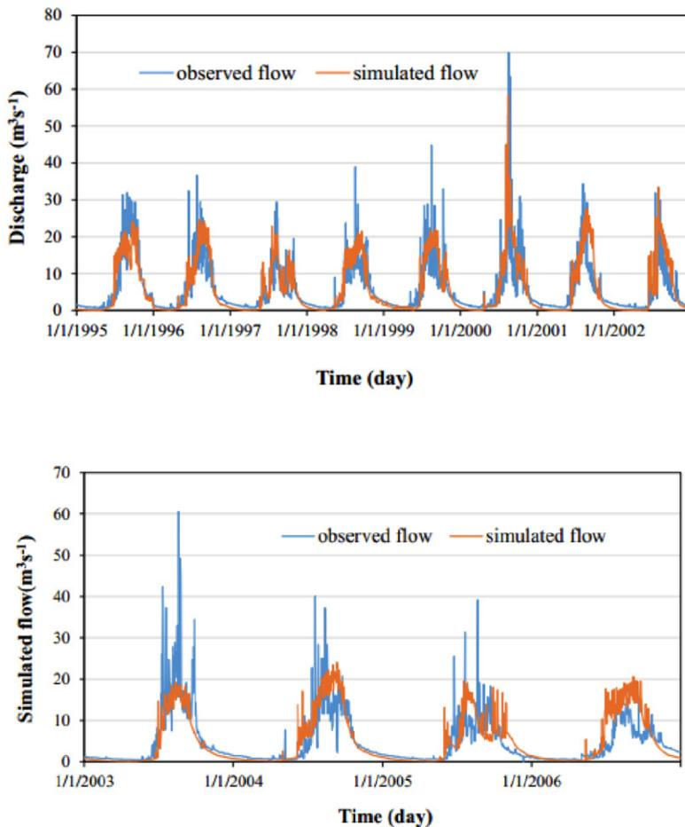
Figure 4 - Daily simulated flow and observed during (a) calibration (1995 – 2002) and (b) validation (2003 – 2006) periods
