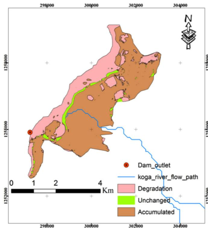
Figure 3 - Sediment distribution in Koga reservoir with sediment extents with reference to the original topography
